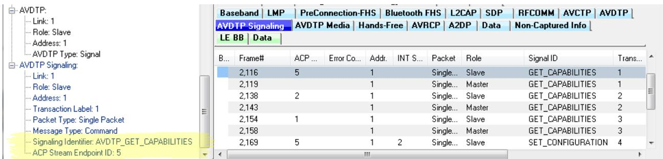
Figure 3 - Frame Display for AVDTP Signaling Frame 2116
