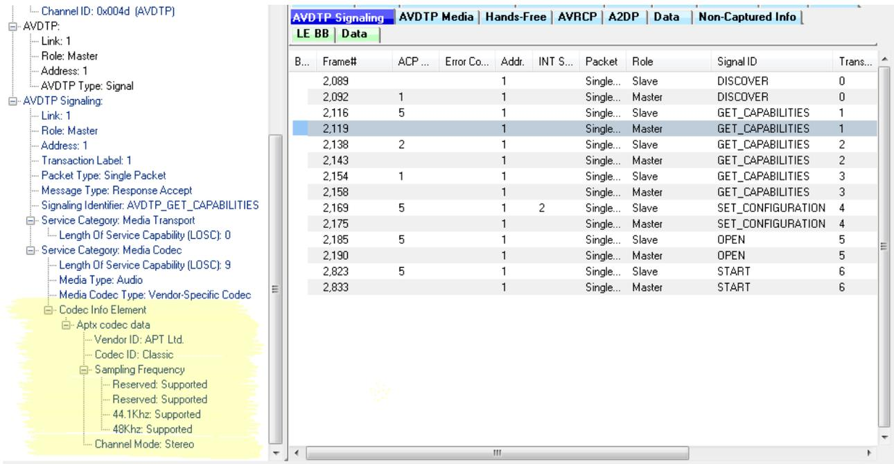
Figure 4 - Frame Display for AVDTP Signaling Frame 2119
