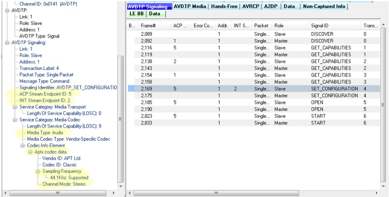
Figure 5 - Frame Display for AVDTP Signaling Frame 2169, SET\_CONFIGURATION
