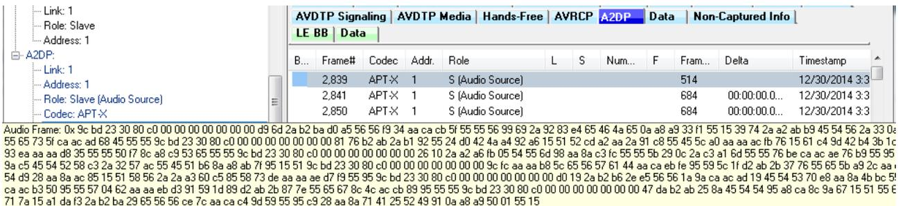
Figure 6 - Frame Display for A2DP Streaming at Frame 2839 with Audio Expanded
